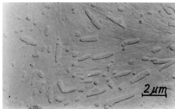
Figure 7 Microphotographs of the films of the PCA-PMAA polymeric mixtures (PCA : PMAA = 80 : 20, mass %).
