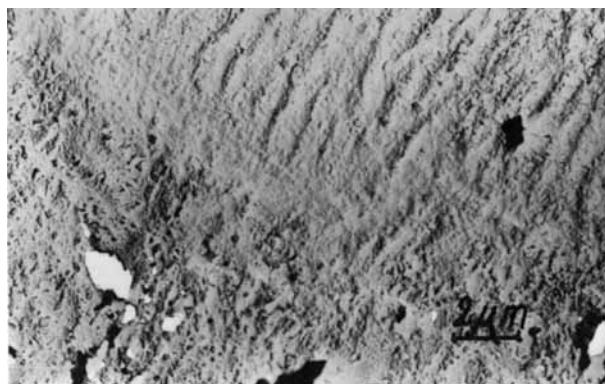
Figure 6 Microphotographs of the cross section of the PCA graft fiber. \omega = 30.7\% .
